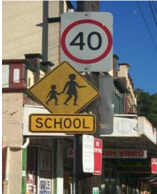
Figure 3: Unacceptable sign clutter
