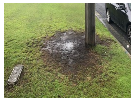
Contamination from a leaking pole transformer
