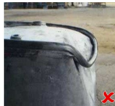
Sharp indents and damage to the rolling hoops or edges are potential leak points
