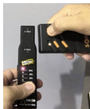
The RF meter is calibrated to the general public limit
