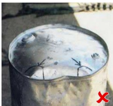
Sharp indents and damage to the rolling hoops or edges are potential leak points
