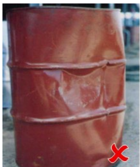
Sharp indents and damage to the rolling hoops or edges are potential leak points
