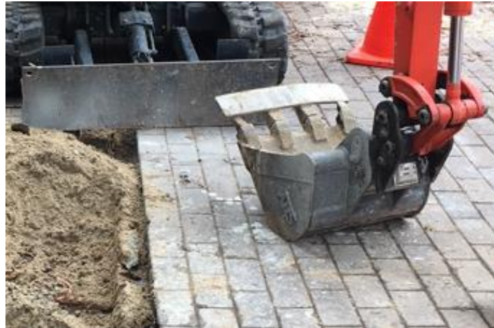
Figure 2: Example of excavator bucket without exposed teeth.
