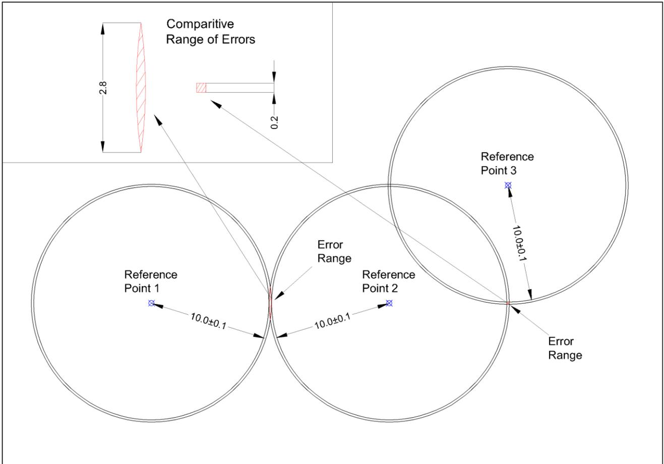
Figure 26 Range of error relates to geometry of reference points
