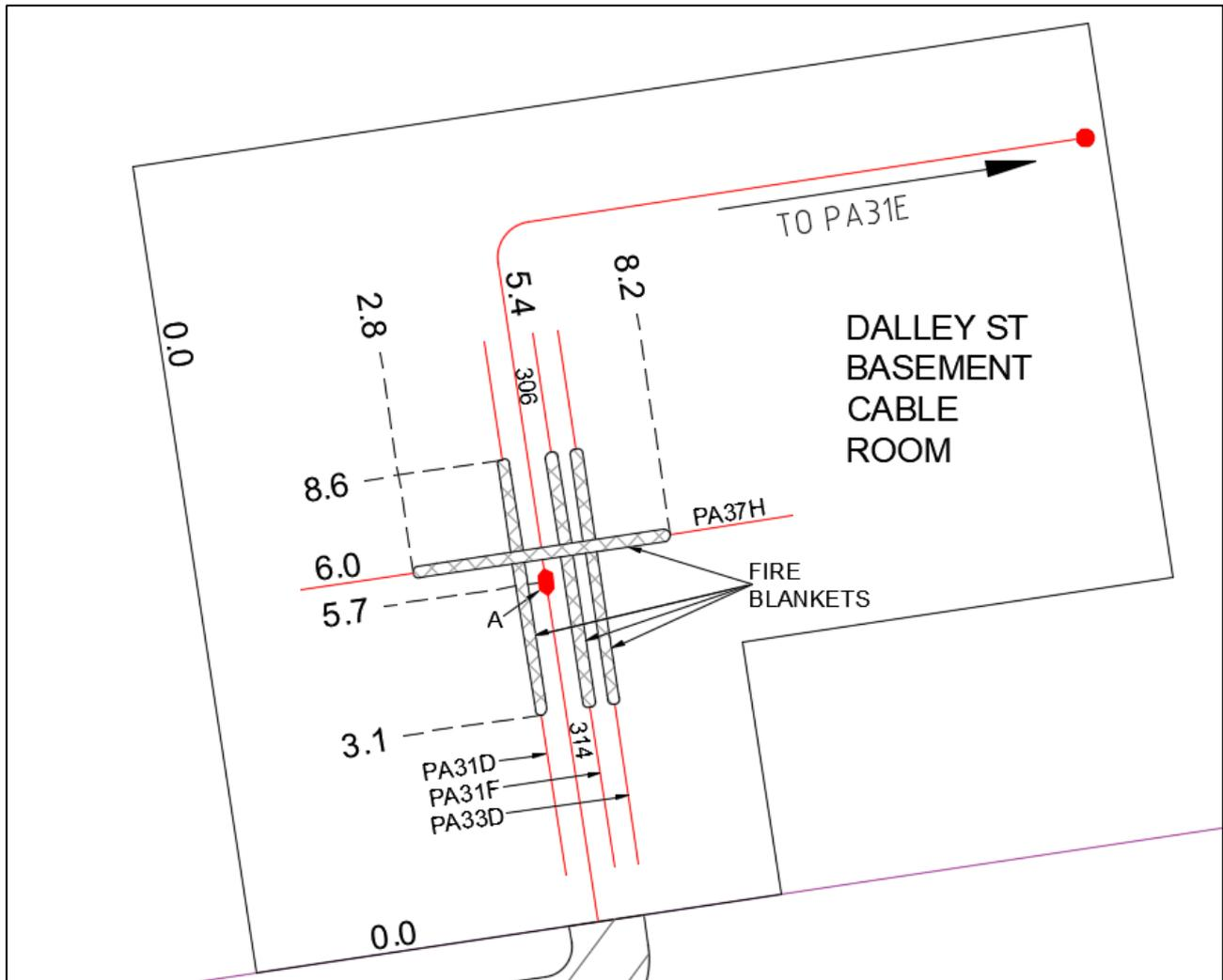
Figure 44 Example recording of fire blankets
