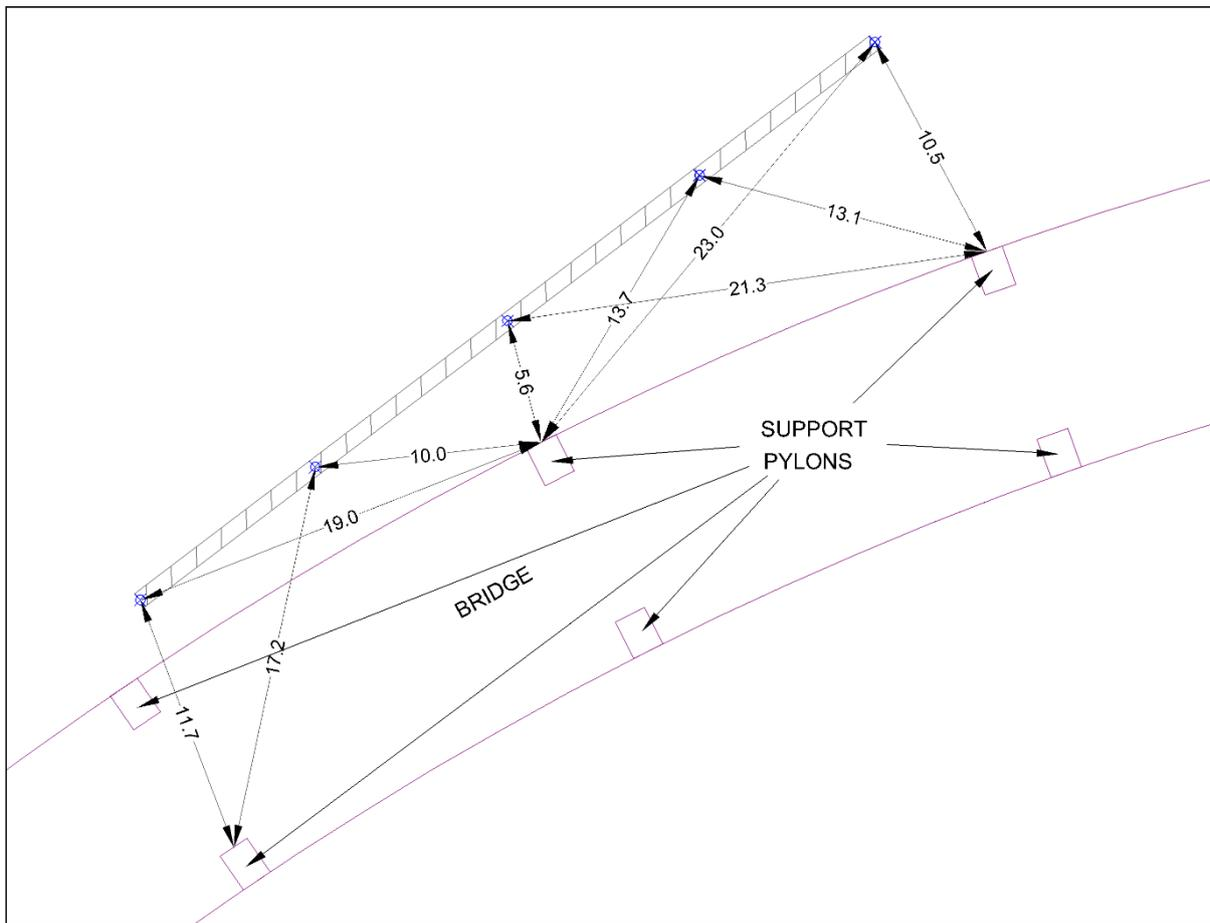
**Figure 25 Ducts measured from bridge supports**
