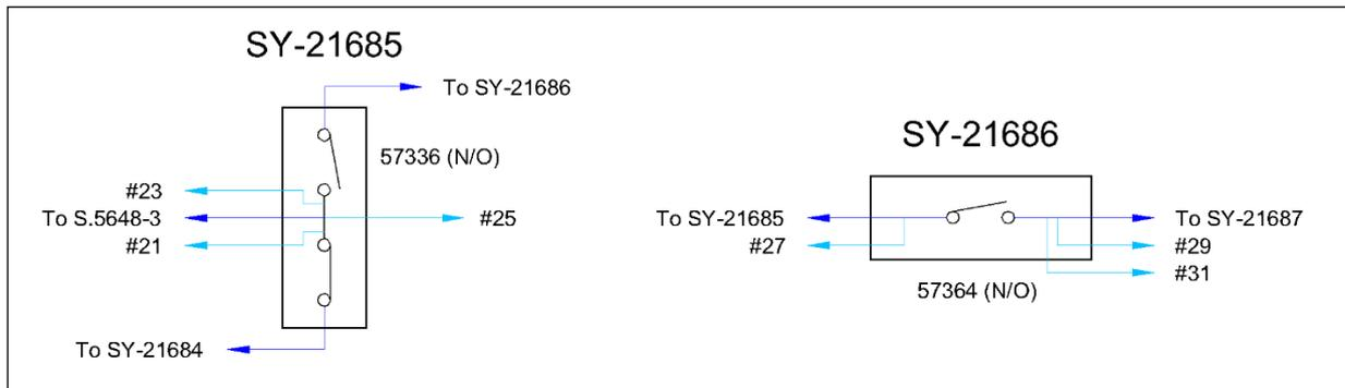
Figure 50 Example of double link and single link pillar diagrams
