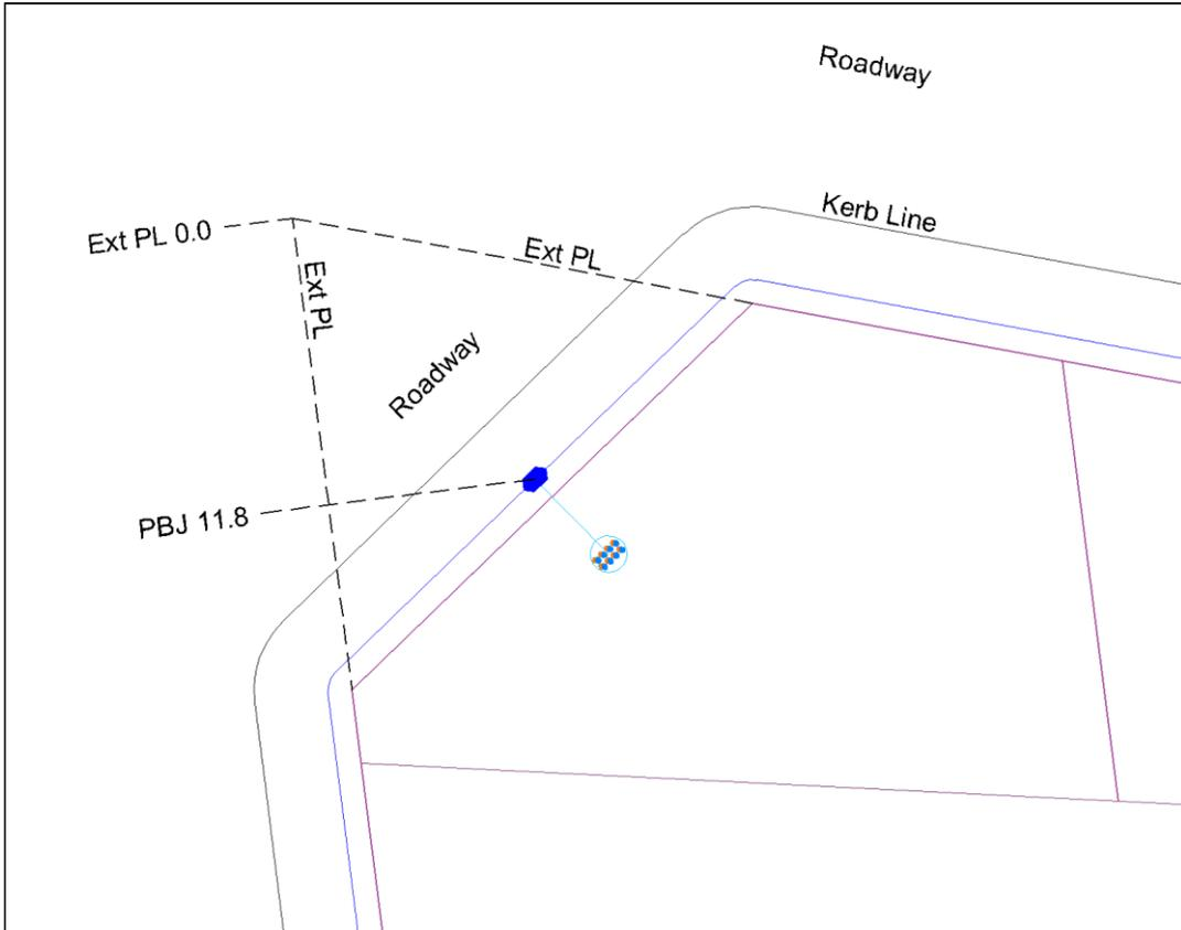
**Figure 23 Extended splay runs into roadway**
