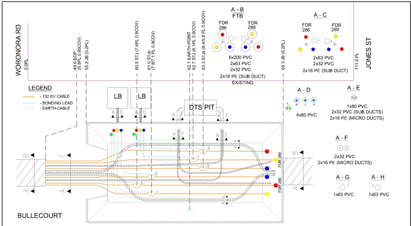
Figure 59 Example of a 132 kV joint bay
