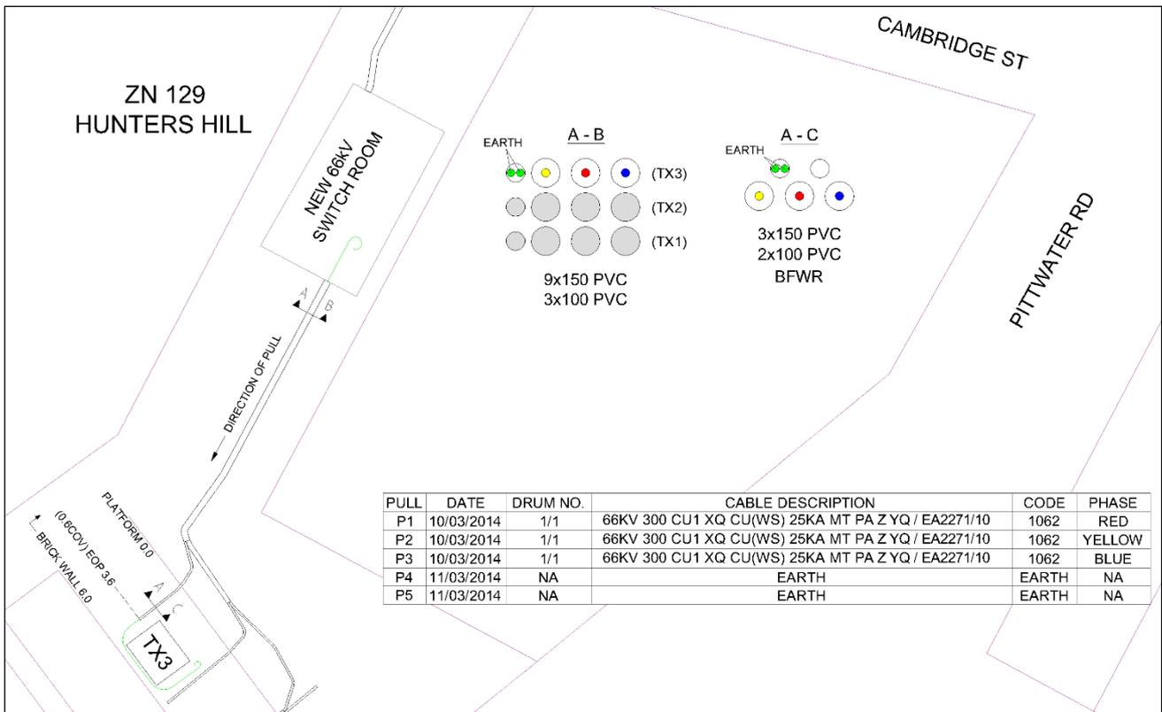
Figure 56 Drum details and direction of pull
