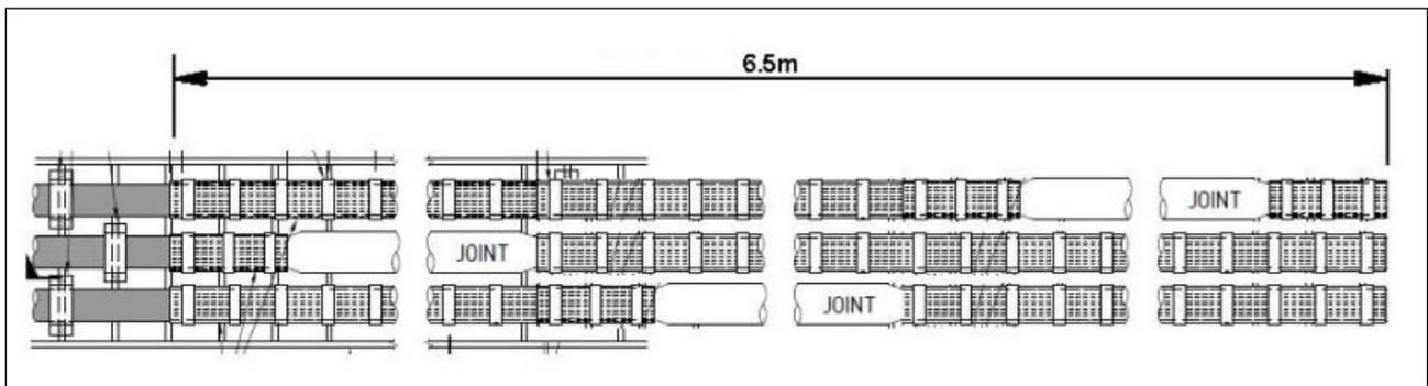
Figure 43 Example of fire blankets wrapping cables in proximity to joints
