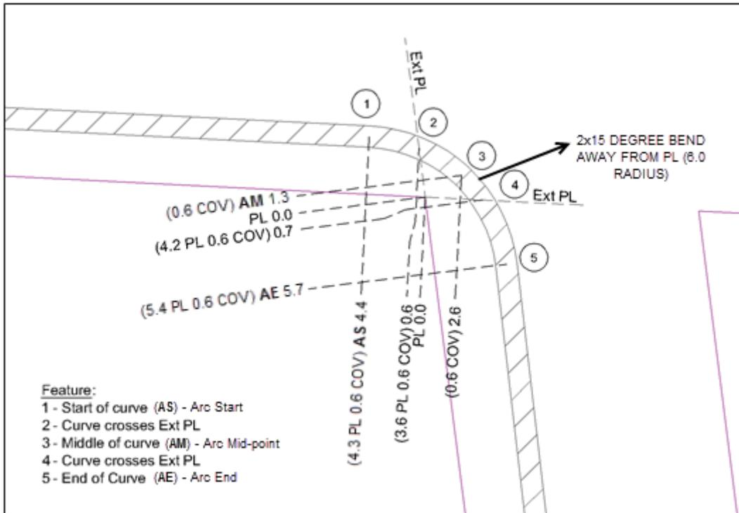
Figure 20 Measuring curves
