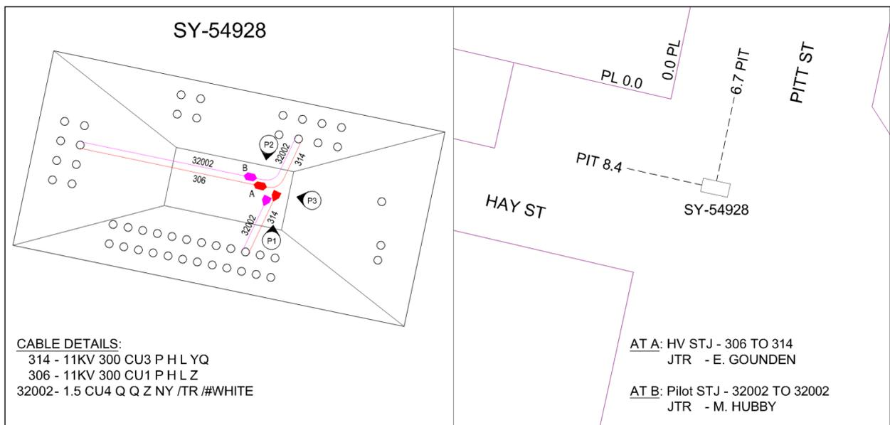
Figure 48 Jointing works in existing pit
