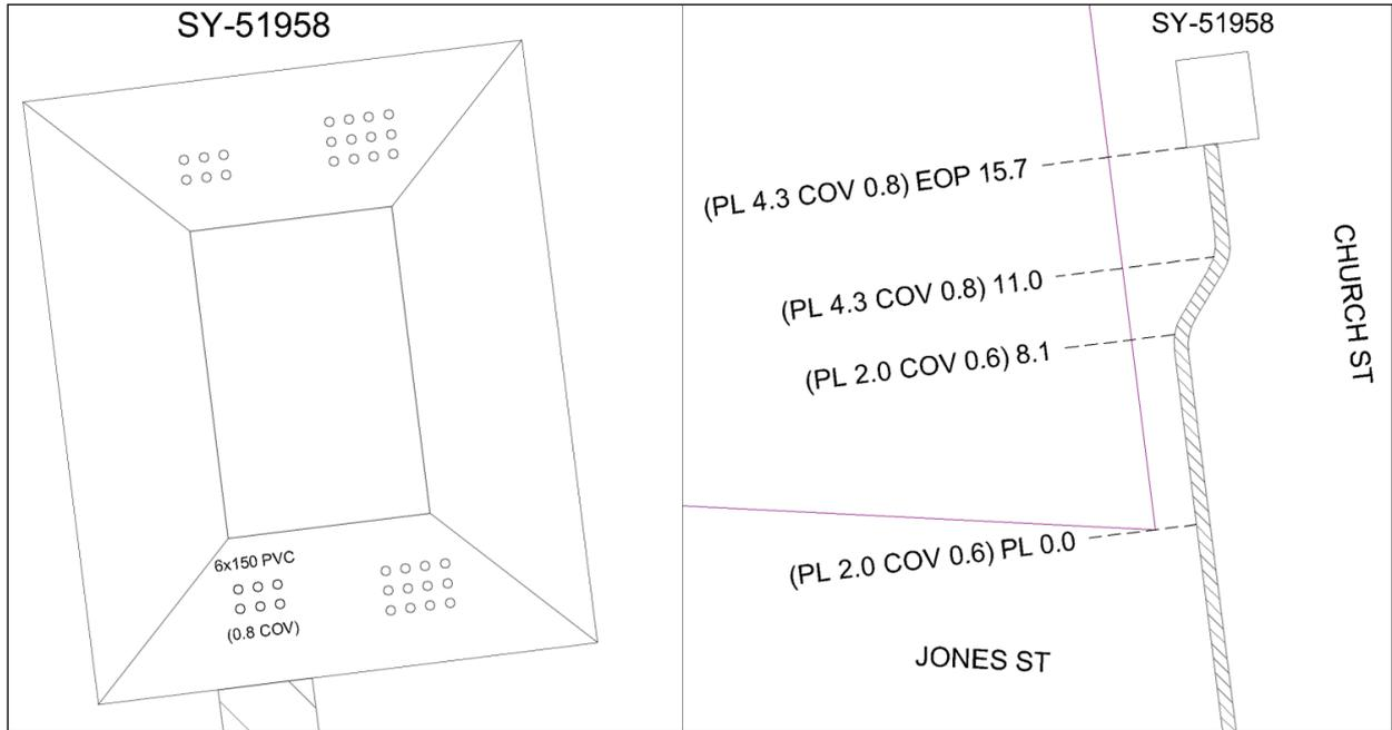
Figure 47 New ducts enter existing pit
