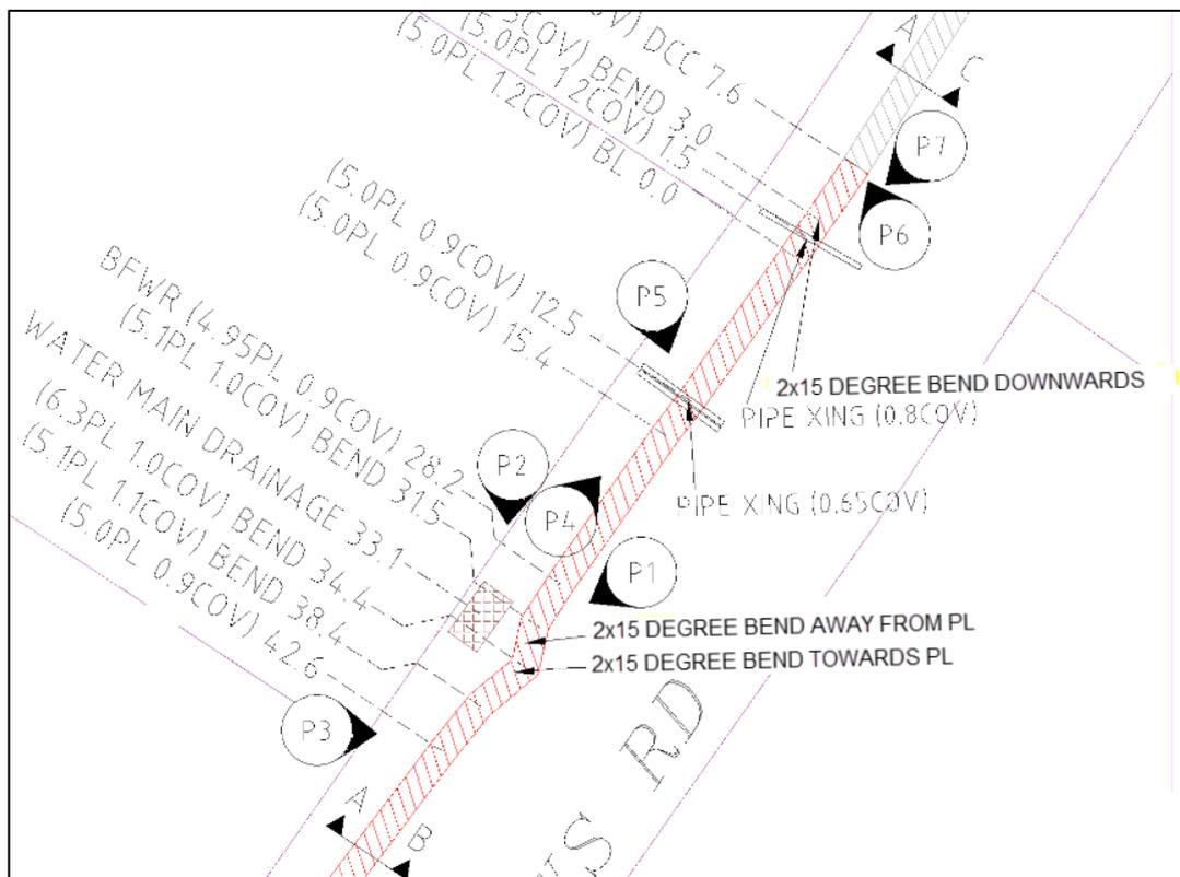
Figure 21 Linear bend changes example
