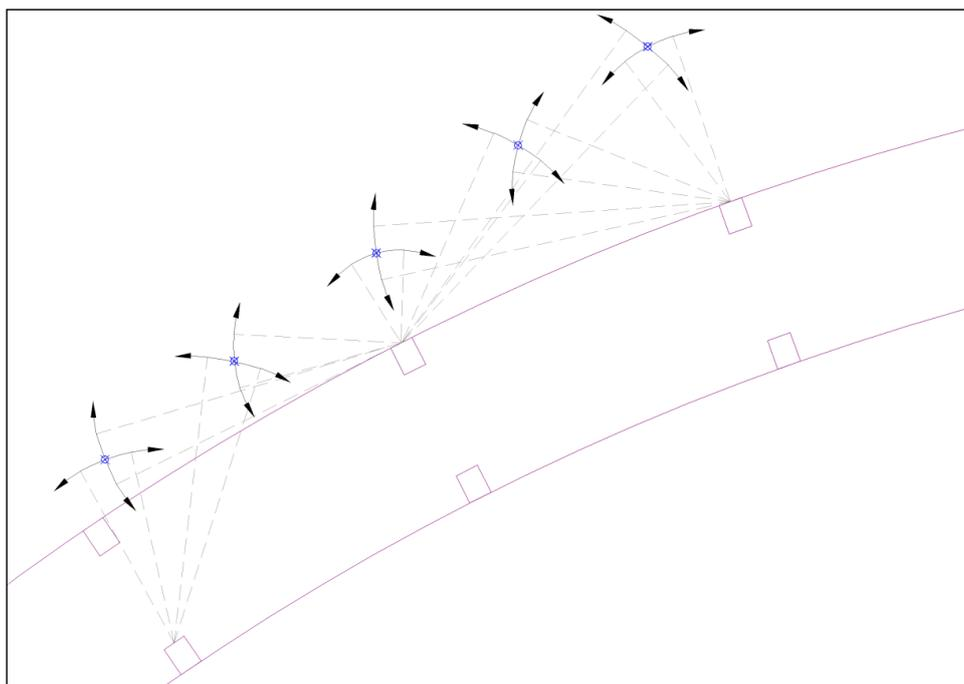
**Figure 28 Intersect arcs to relocate recorded positions**
