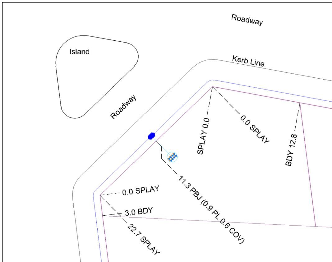
Figure 24 Face of splay used as baseline
