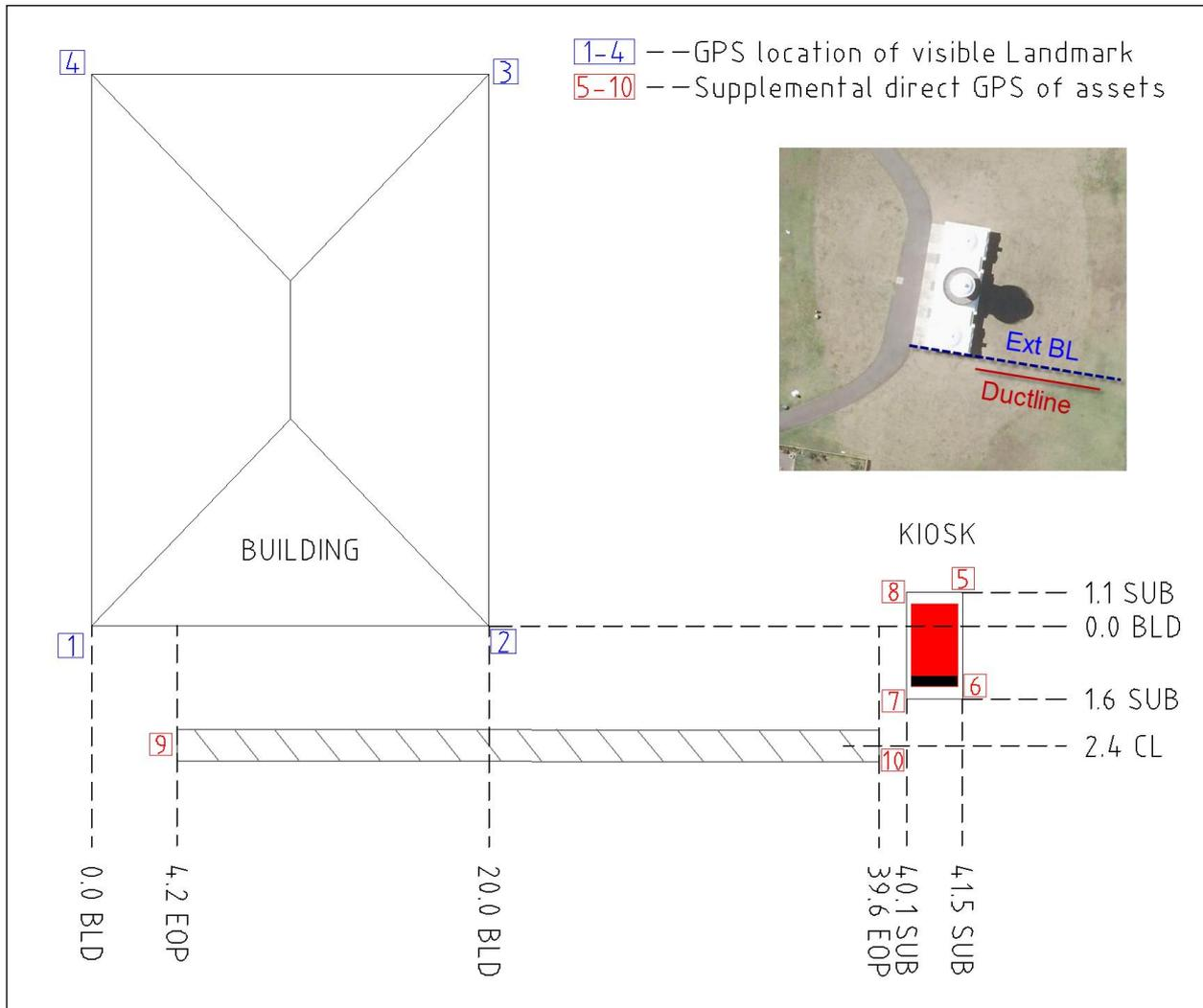
Figure 13 First choice – measured from visible landmark
