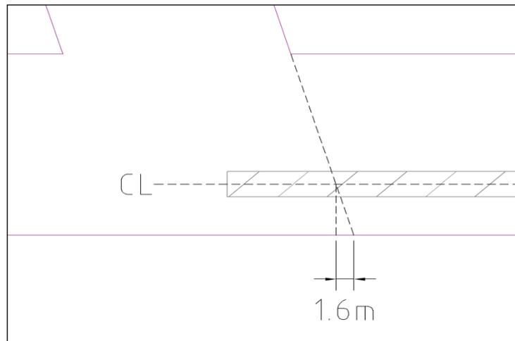
Figure 18 Measurement error when PL not extended properly
