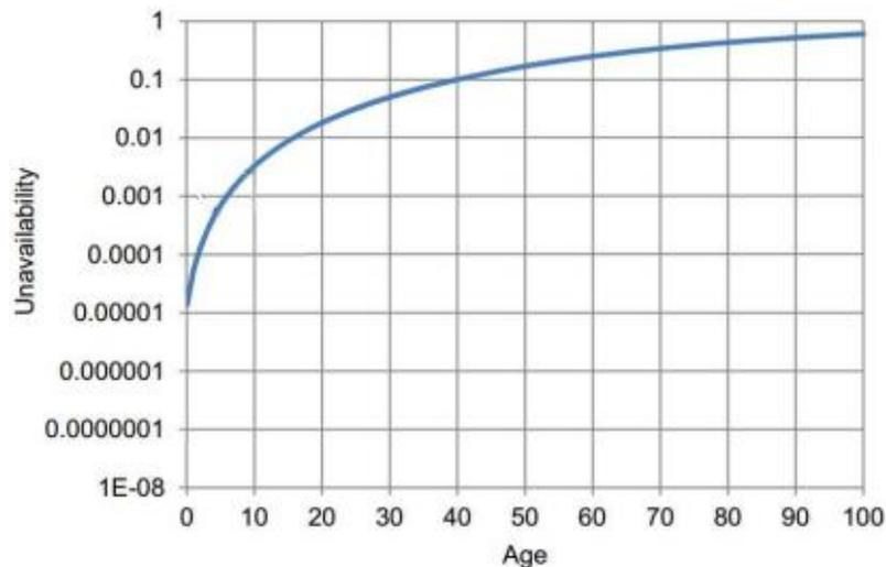
This model is also based on the relationship between the condition of a cable and its age. The Crow-AMSAA model shows that the availability of fluid-filled cables is expected to decline significantly if the cables are retained past an age of 50 years. Ausgrid considers this methodology is consistent with industry practice. A detailed discussion of the probability of failure and asset availability is provided in Appendix D.
