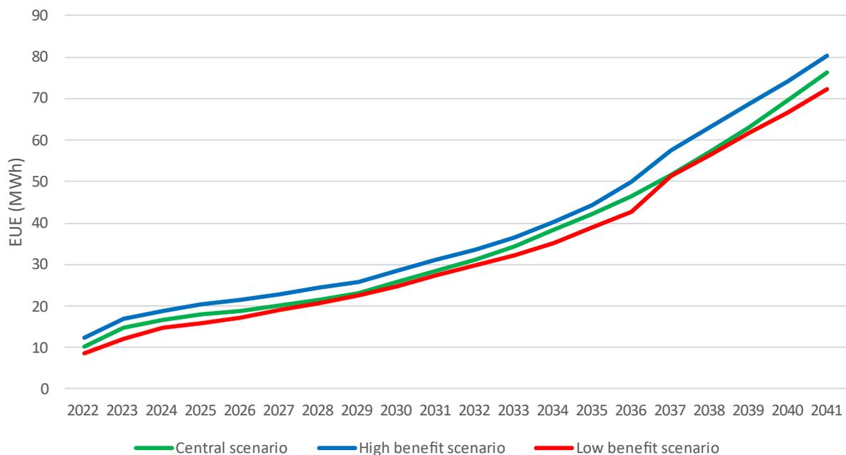
Ausgrid has developed a model to quantify the failure parameters (probabilistic distribution of outage frequency and duration) of each cable, relative to its observable condition. The failure model is applied to a probabilistic model of the network and the demand it is supplying, to estimate the long-term average amount of annual energy that is beyond the technical capability of the degraded network and therefore cannot be supplied given the expected reliability and loading levels.
