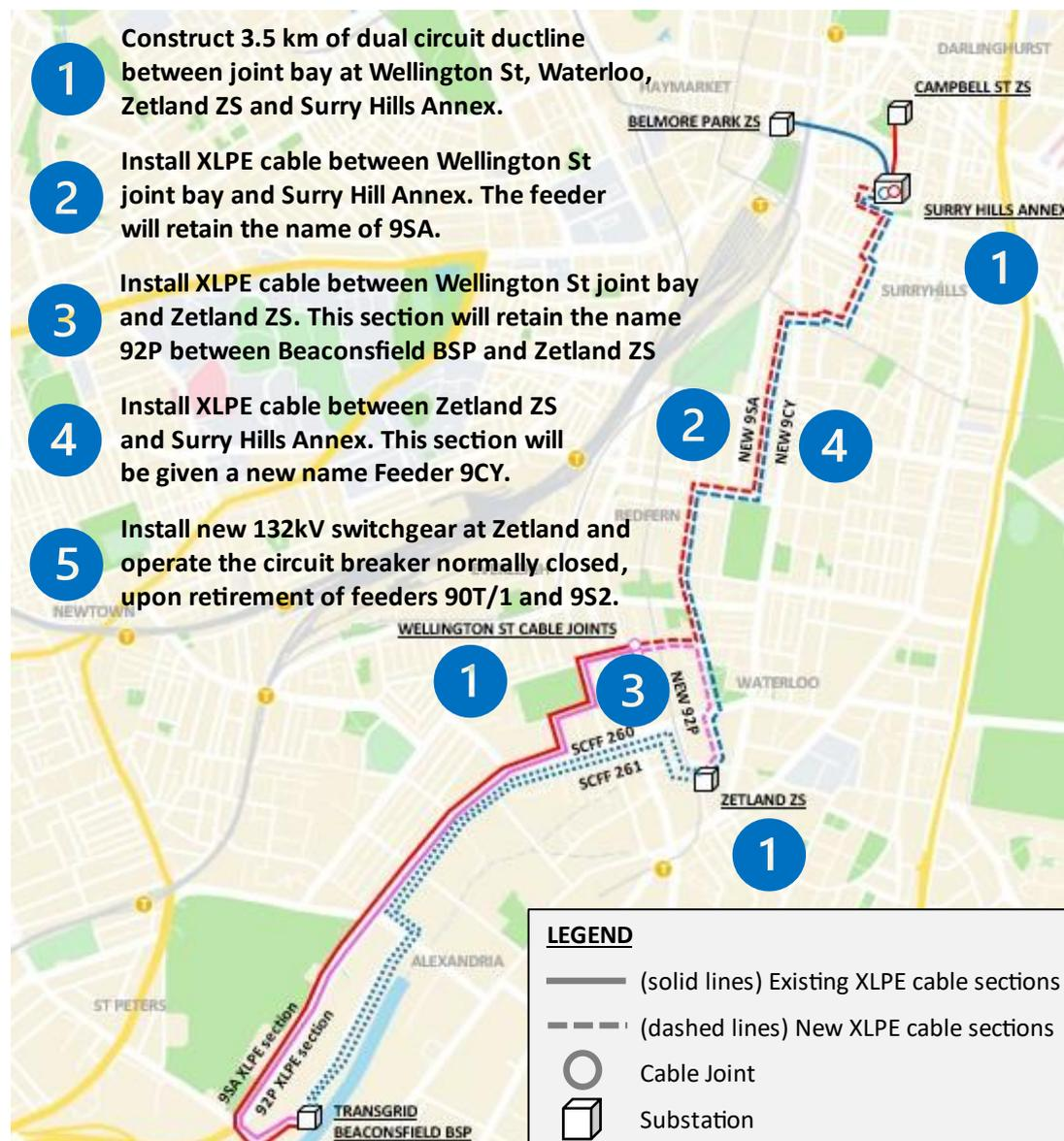
Figure 3-3 below illustrates the existing and proposed network arrangement at Zetland ZS under this Option 2.
