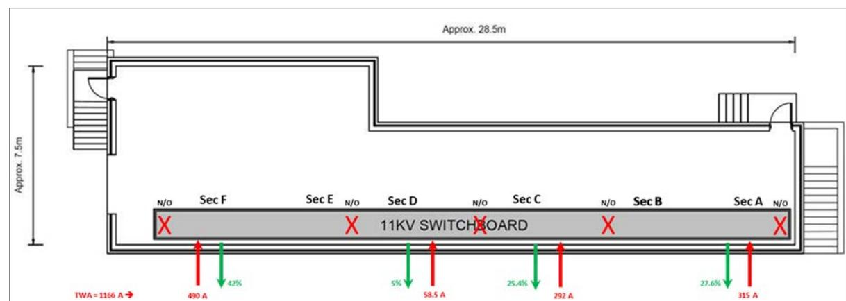
**Figure 11** Loading scenarios for new 11kV switchboard that can be used for EMF calculations
