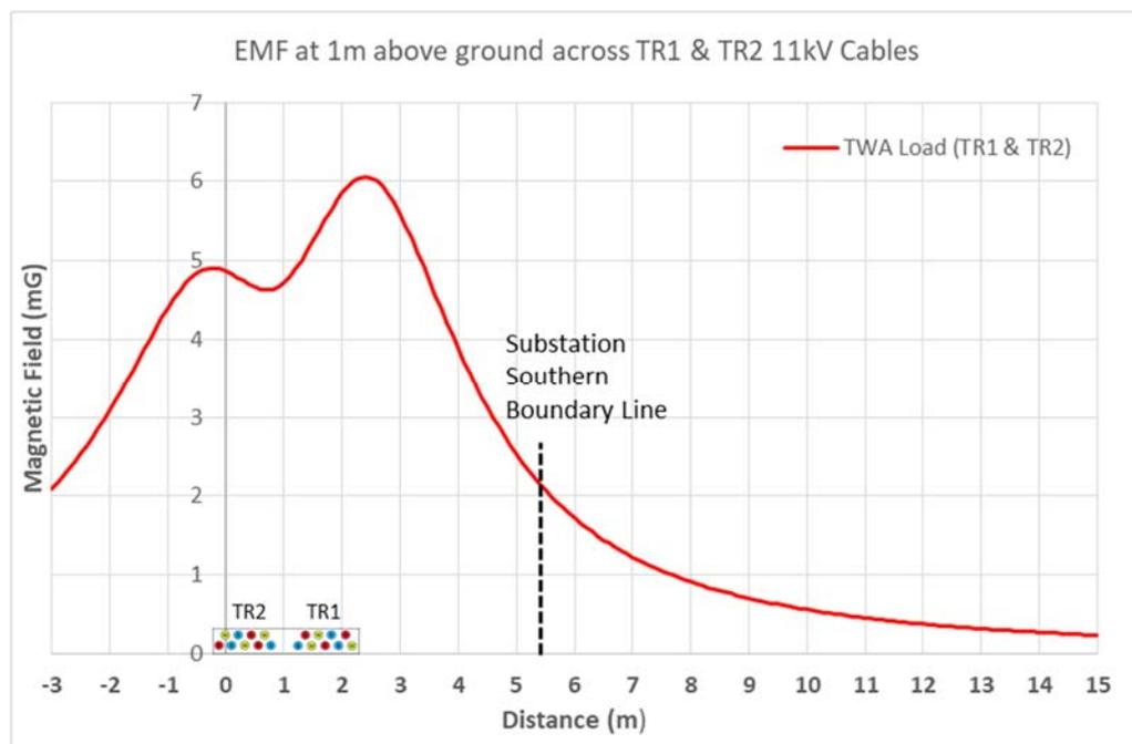
**Figure 8 EMF profile calculated at 1m height across the 11kV cables of TR1 and TR2 transformers in the southerly direction.**
