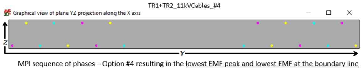
**Figure 6 Phase arrangement which results in the lowest magnetic field.**
