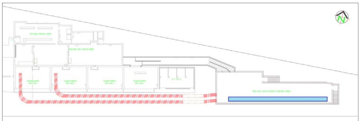
**Figure 2 Plan view of Concord Substation with 2 sets of underground 11kV transformer cables connecting Transformer 1 and 2 to the new 11kV switchboard**
