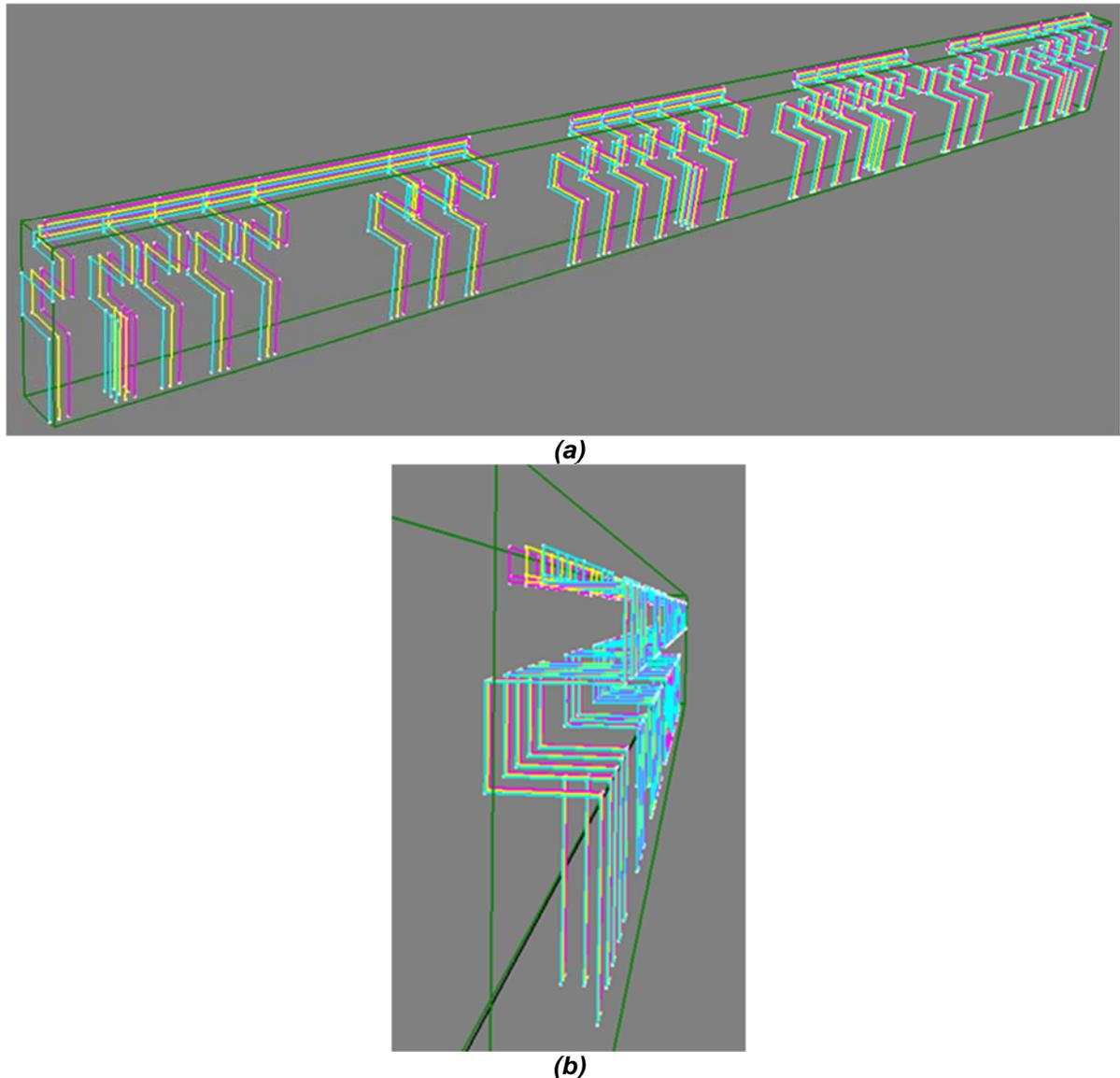
**Figure 12**      **3D computer modelling image of new 11kV switchboard**
