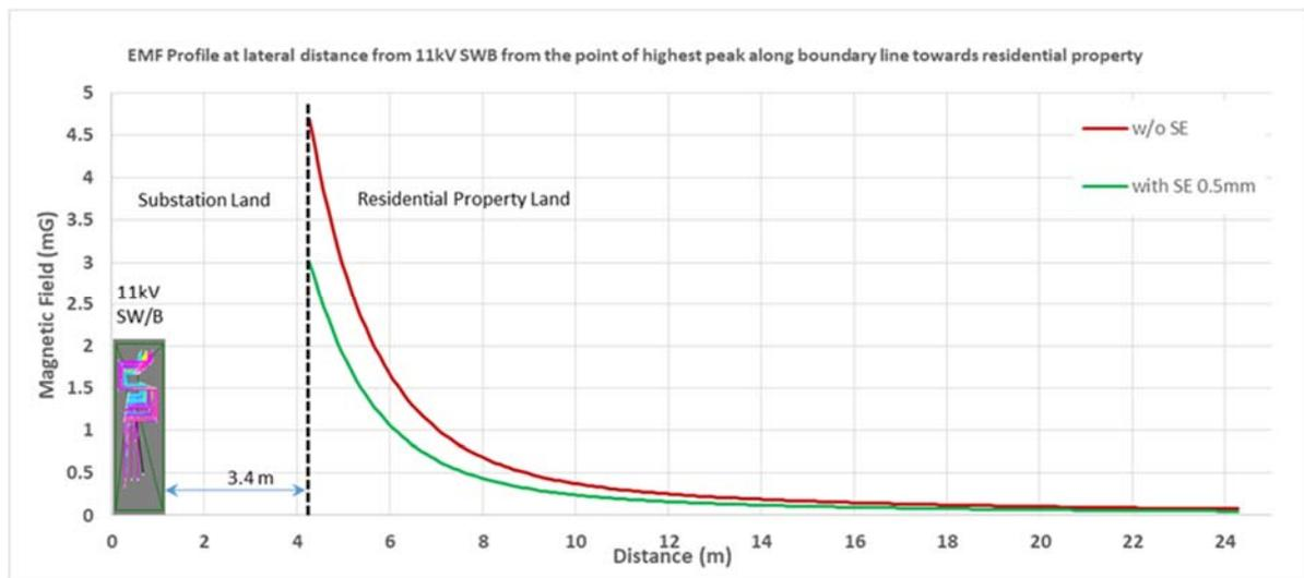
**Figure 14** EMF profiles at lateral distance from 11kV switchboard from the point of the highest peak of profiles shown in Figure 16.
