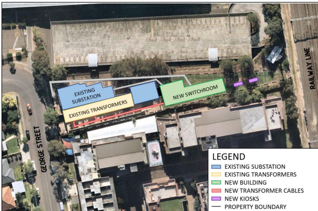
**Figure 1 Proposed new works within Concord Substation**
