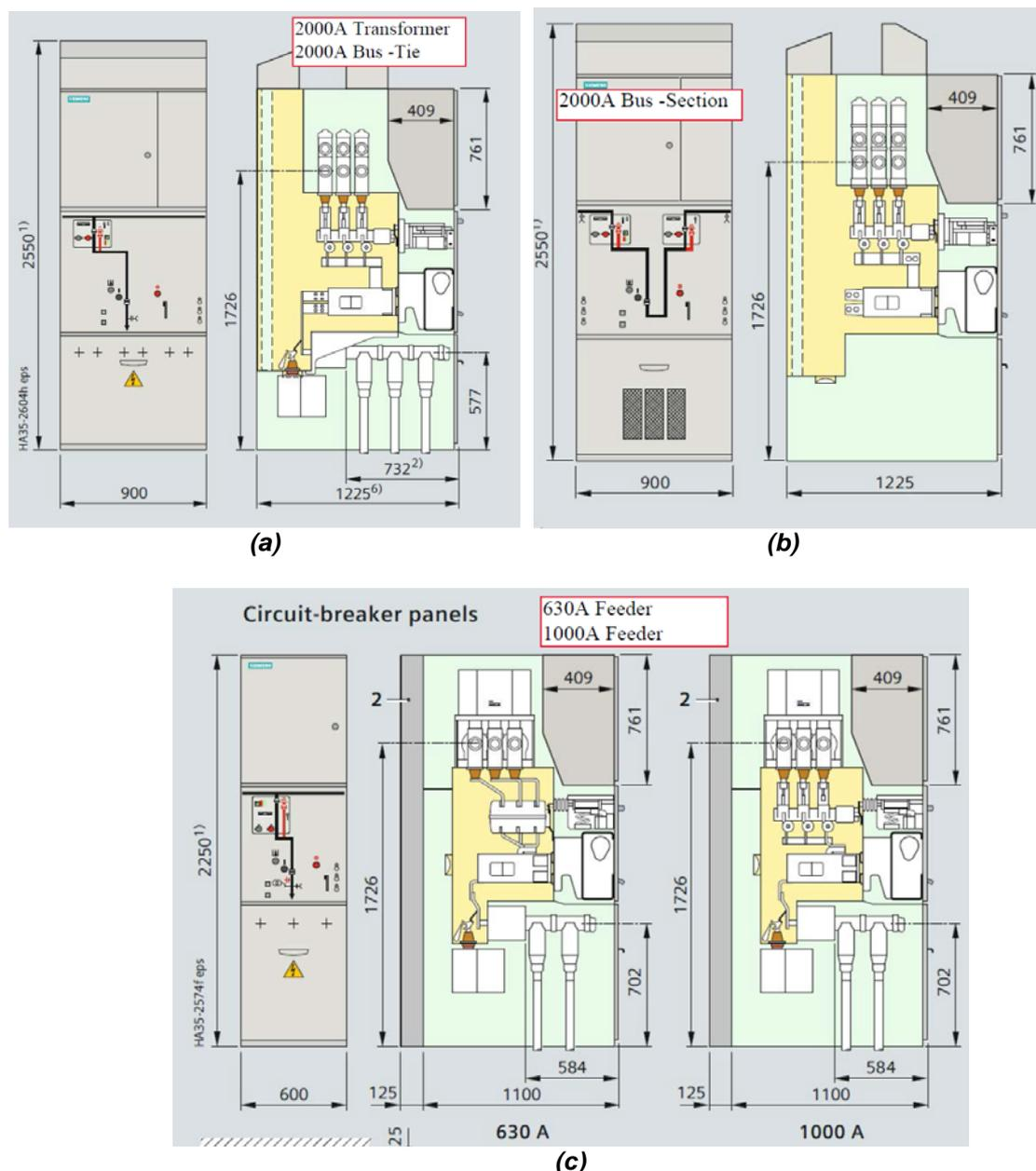
Figure 9 Transformer / bus-tie compartments (a), Bus-Section (b) and Feeder compartment (c)
