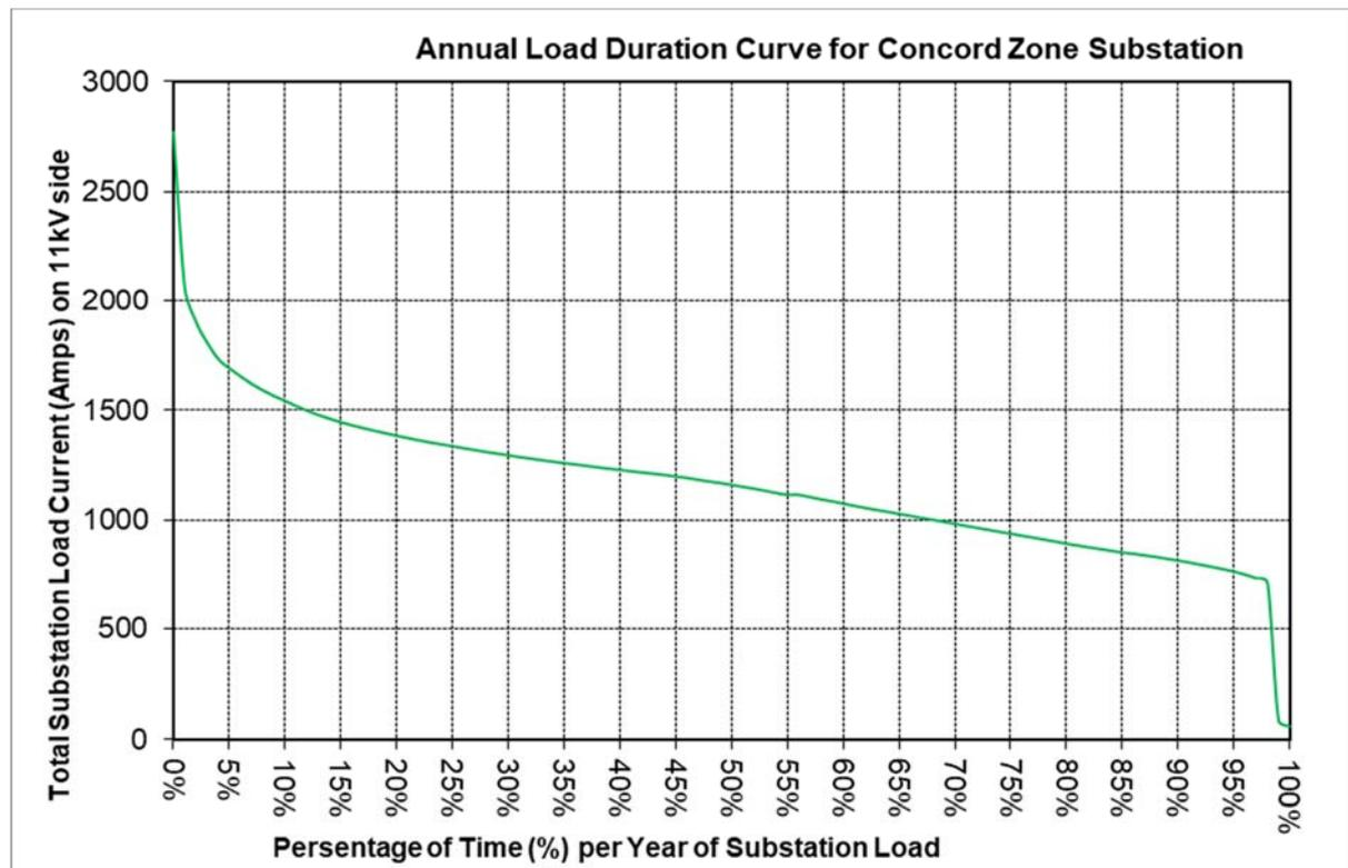
**Figure 10** Extrapolated annual load duration curve for Concord Substation for 2022-23
