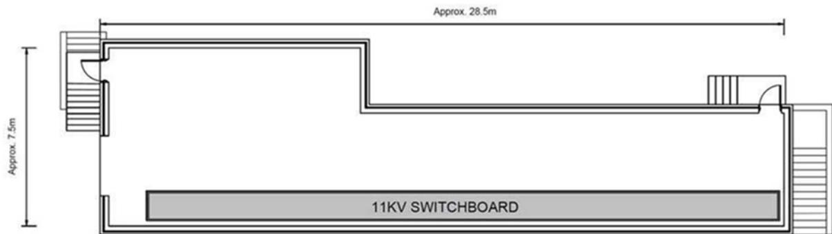
**Figure 4 Proposed new 11kV switchboard**
